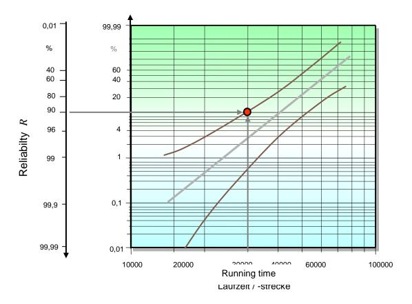
$P_A$  was originally introduced as the probability for the failure of a test specimen. The prerequisite is that these test specimens are a random sample of a "population". A conclusion is drawn based on the samples where the definition corresponds to the confidence bound of the illustrated Weibull plot.
