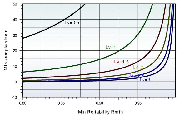
As illustrated, the prerequisite for this scope of random samples is that no failures occur.
